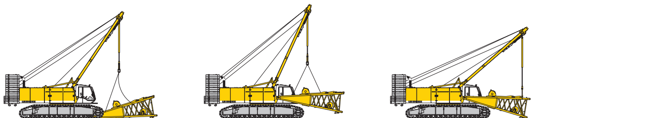
Unloading and assembly of boom foot
